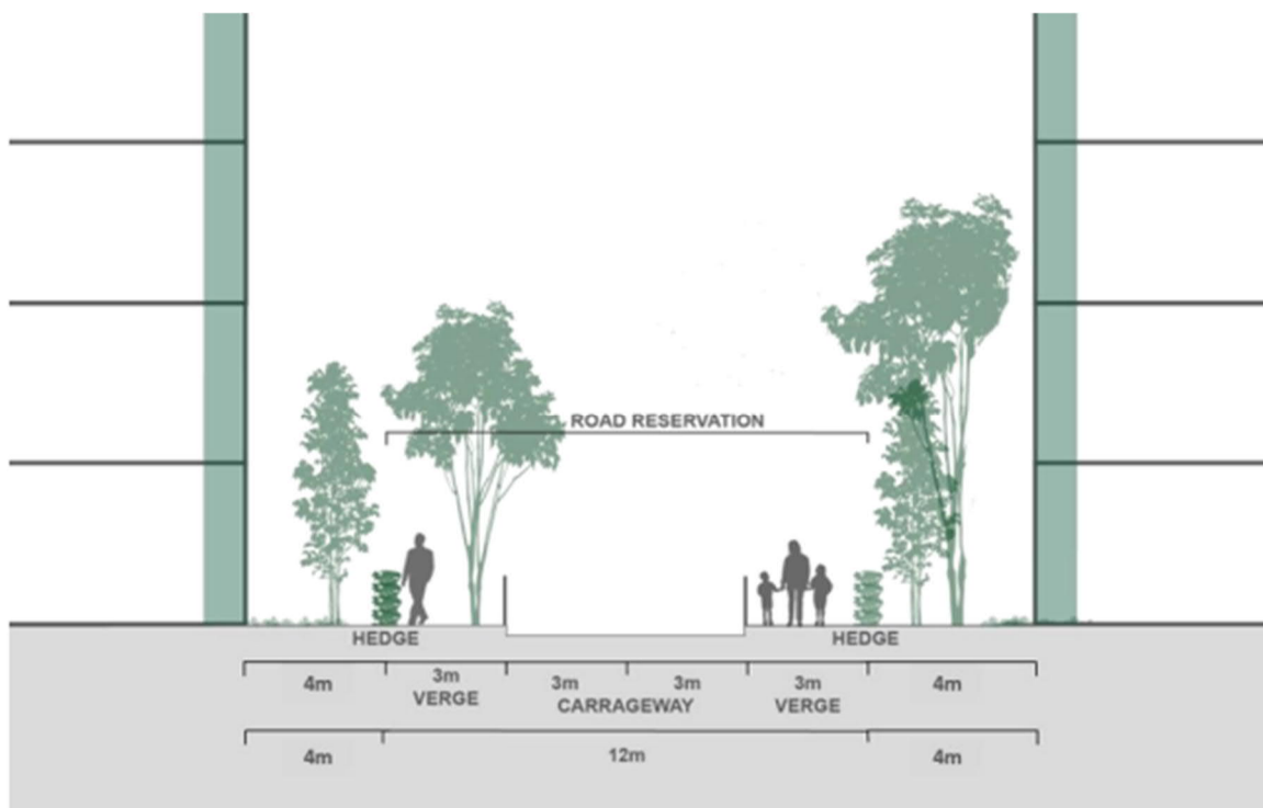
Figure 9: Typical section of new DCP Road adopted in the LCDCP
